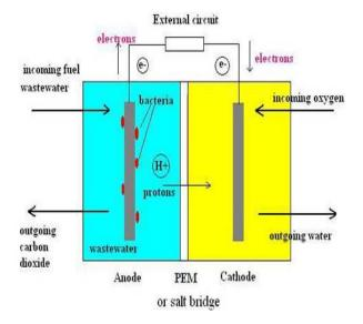
Fig: 9. Schematic diagram of two-chambered MFC.
