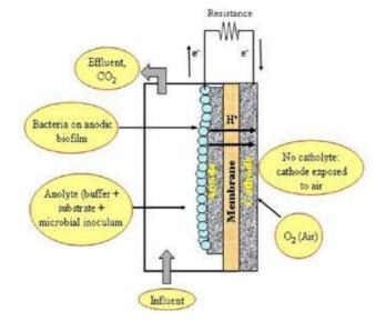
Fig. 8: Schematic diagram of single-chamber MFC (©Pant *et al.*, 2010).
